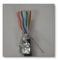
6. Using wire cutters, trim the end of the wires evenly to ensure a straight surface to insert into the *TOUGHCable Connector*.
