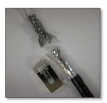
3. Carefully fold back the drain wire numbered 0 in the Cable Wiring Specification (T568B).
