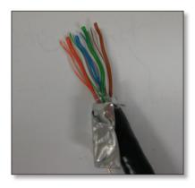
Fold the foil shield back up towards the exposed wires; leaving roughly half the distance exposed while covering the bottom half with the foil. Fold under or tear away any excess foil. Using wire cutters, trim the end of the wires evenly to ensure a straight surface to insert into the TOUGHCable Connector.
