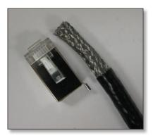
Carefully remove the twisted wire shielding covering the drain wire and foil shield.
