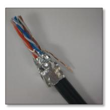
4. Cut or tear away the the clear plastic wrapping around the twisted pair cable and untwist the wires that are exposed.
