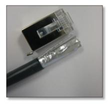
2. Carefully fold back the foil shield to expose the drain wire and twisted pair cable.
