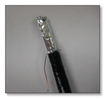
4. Carefully fold back the foil shield to expose the clear plastic wrapping around the twisted pair cable.
