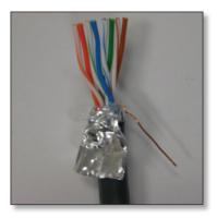
Fold the foil shield back up towards the exposed wires; leaving roughly half the distance exposed while covering the bottom half with the foil. Fold back any excess foil.
