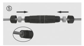
5. Lock the two waterproof plugs on the cable, then put them into the end of the long tube. **Note:** The plug is engraved with the word "waterproof" on one side outward.
