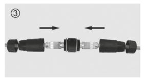
3. Insert the patch cord into the both ends of the RJ45 coupler.
