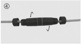
4. Screw the long tube tightly onto the RJ45 coupler as guided in themanual.
