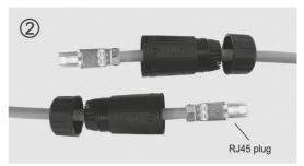
2. Pass the two cables through the end covers and the long tubes respectively.
