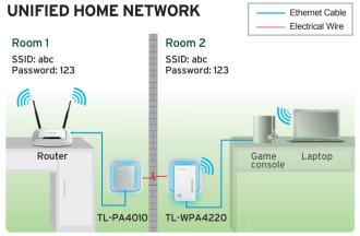
\*The Powerline Adapters need to be connected in the same electrical circuit.
